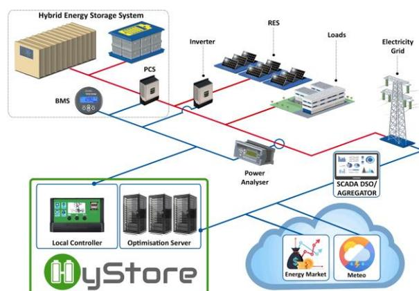
Figure 4. Block scheme of the *HyStore* hybrid energy storage management system
