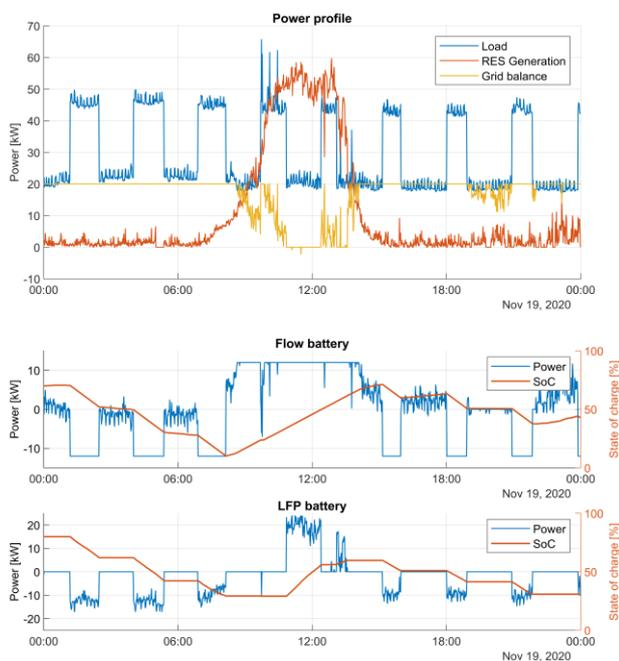
Figure 3. Daily profiles of a flow-lithium hybrid system
